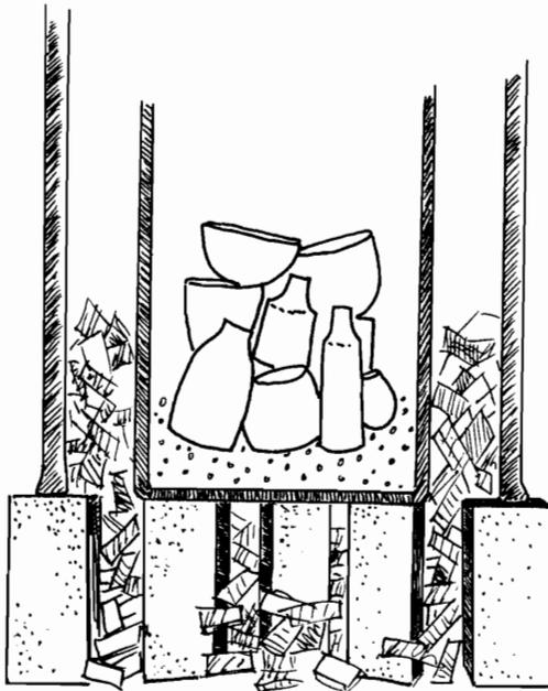
Figure 13-28. Double drum kiln.
