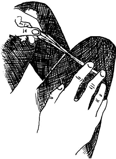
Figure 10-5. Drafting and hand rolling fibers.
