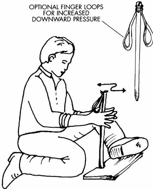
Figure 4-6. Using a hand fire drill.
